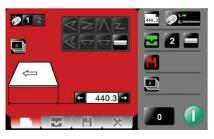
Using the screen is simplicity itself. Key in the sheet length (popular sizes are pre-set), touch the fold type for the finished product (letter, gate etc) and press the green button. The AutoCreaser Pro 50 will automatically calculate
